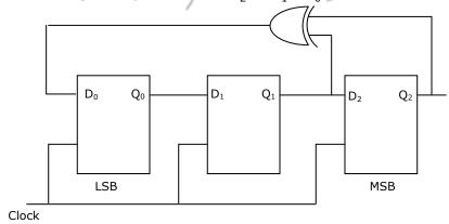
Which one of the following is the correct state sequence of the circuit?
